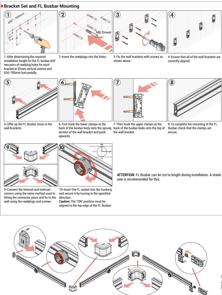
ATTENTION: FLD busbar and cover can be cut during installation. To do this, it is recommended to start from corner mounting points and use of motorized circular saw for less casualties and easy installation.
