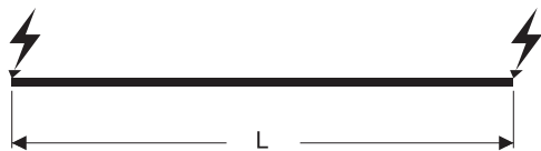
2 feeding points from the start points, L_t = L/4
