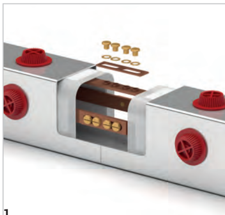
1 Connect the coppers with an joint unit.
